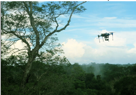
A lightweight 3D Robotics Iris multirotor drone is used to capture canopy structure and spectral reflectance rainforest canopy during the April 2017 workshop in the Amazon, led by Patrick Meir.
