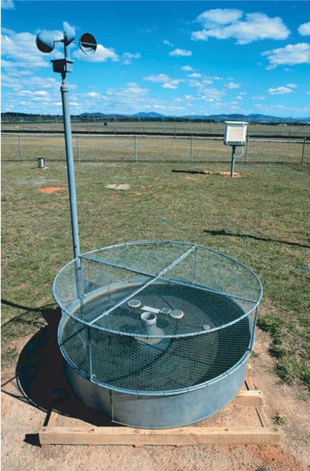
Fig. 1. The Class A pan evaporimeter at Canberra Airport. This pan is one of about 300 maintained by the Australian Bureau of Meteorology throughout Australia. Water in the pan is replenished and measured daily along with the minimum and maximum water temperature and precipitation. Australian pans are fitted with bird guards that reduce the daily pan evaporation rate by about 7% (van Dijk 1985).
